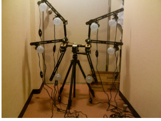
Figure 6. Measurement system “Photometric Wing” used for the tumulus.
