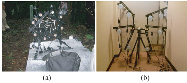
Fig. 20 Measurement system used for Segonko Tumulus: (a) Photometric Diamond, and (b) Photometric Wing.
